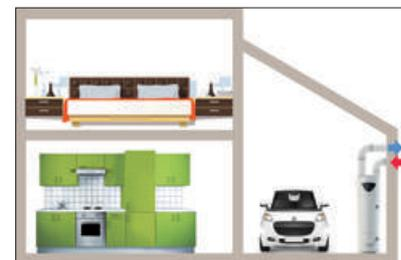
AIR EXTÉRIEUR AVEC GAINÉ POUR NE PAS REFROIDIR LA PIÈCE (HORS VOLUME CHAUFFÉ)
